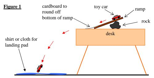
The basic plan is that we will release the car on the ramp; the car will roll down the ramp and off the desk, flying through the air and hitting the floor. Based on measurements of the ramp and of the desk, we will try to calculate where the car will land using some equations from the physics syllabus. In terms of the illustration below, we will measure x and y and thereby calculate z:
