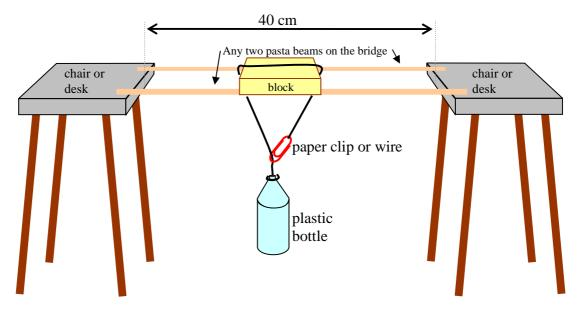
The reason for hanging the weight from the block (rather than attaching the string directly to the pasta) is to allow the weight to be spread across separated beams without causing beams to be pulled together horizontally.
